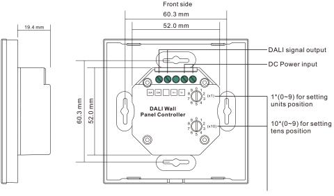
Rotary switches for setting start DALI address number (0-63), the number equals to tens position plus units position
